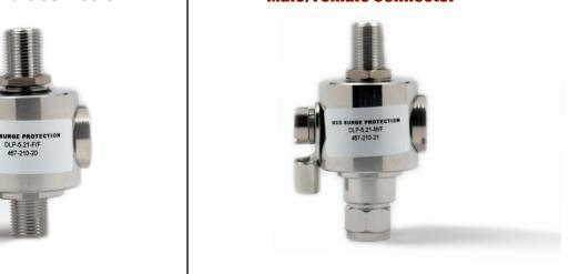
Costly digital communications are the norm and protecting equipment like set top boxes, modems and flat panel TVs is vital to ensure uninterrupted operation. The DLP-5.21 protects cable input circuits in this equipment, such as tiny surface mount ICs and conductors that carry the signals. Sensing overvoltage events, the protector safely diverts surges away from sensitive equipment. Installs in minutes using type "F" connectors. Covered by MCG's 20 year "No Nonsense" warranty.
