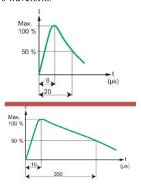
The waveform above the red line is the 8/20. It roughly agrees with the results of many studies and measurements of lightning that have been made by meteorologists and lightning scientists throughout the world.
