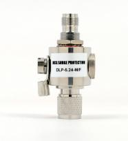
The DLP-5.24 is a high bandwith protector used to protect many 50 Ohm based coaxial systems up to 780 Watts power. Typical applications are broadband systems, two-way radios, cellular systems, wireless LAN, coaxial cables, and amateur radio equipment. The DLP-5.24 uses a rugged gas discharge tube which bypasses the surge to ground thus protecting downstream equipment. Installs in minutes indoors or outdoors, uses TNC connectors, and is covered by MCG's 20-year, "No-Nonsense" warranty.
